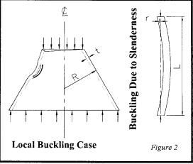
the plate and R is the radius of curvature of the member measured perpendicular to the point under consideration to the axis of rotation.) When t/R is between 0.0035 and 0.125, buckling is in the inelastic range; and for values of t/R greater than 0.125, buckling is in the plastic range.
