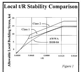
dard has been modified to allow higher stresses in compression than was formerly permitted by the D100-84 standard due in part to more restrictive construction tolerances. Ad-
