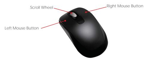
The USB mouse is the primary and recommended method for controlling the system. Listed below are the various functions that the mouse buttons perform.
