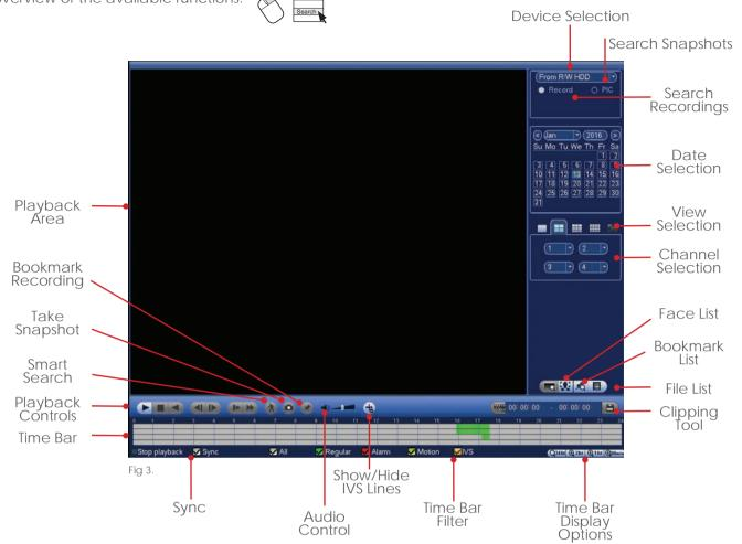
To playback footage from a specific time period, use the **left** mouse button to select the date, view type and camera channels. The timebar should display available recordings for the chosen cameras and date. To start playback double click the **left** mouse button on the desired area of the time bar.
