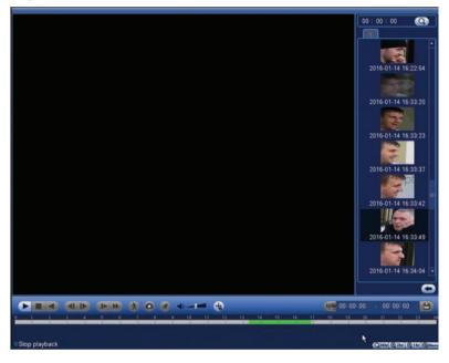
A list of snapshots should of appeared on the right side of the screen, to browse the snapshots scroll up and down. To playback a snapshots event, double click the **left** mouse button on the snapshot.
