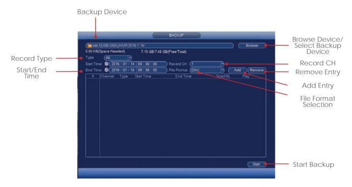
With the Backup menu displayed it is possible to add specific dates/times, camera channels and record types. Mutliple backup entries can be created so that different incidents can be backed up simultaneously.
