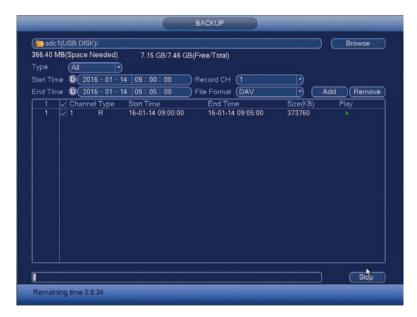
During the backup process a progress bar is displayed with an estimated completion time. Once the backup is finished a Backup Completed message will be displayed.
