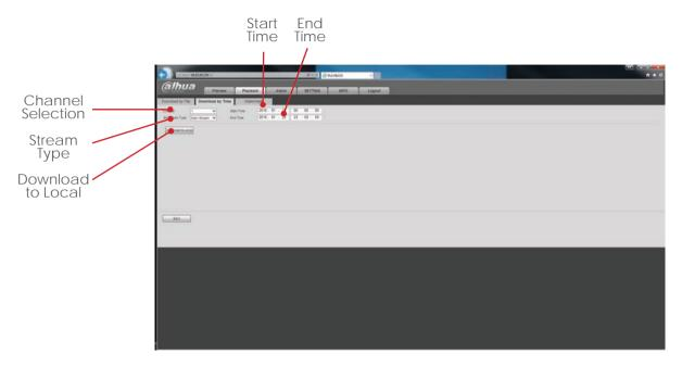
To copy a specific time range to the computer first select which channel to copy using the **Channel Selection** box.
